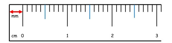
This gap is there to allow the rule to be used should the edge or end be chipped, damaged or worn away. However, as an Engineer's rule is made from steel, the end should not be damaged, so the end of the rule is the point where you will take all measurements from.
