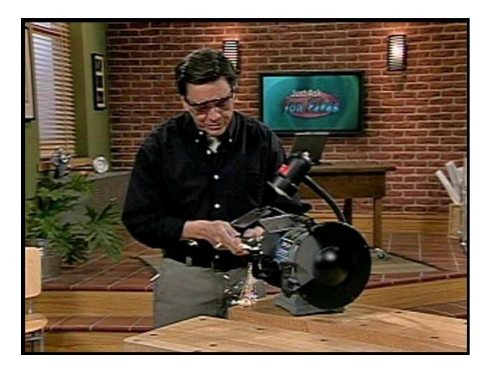
The chisel is being held against the tool rest, with both hands to ensure a safe grip and is standing at right angles to the grinder.
