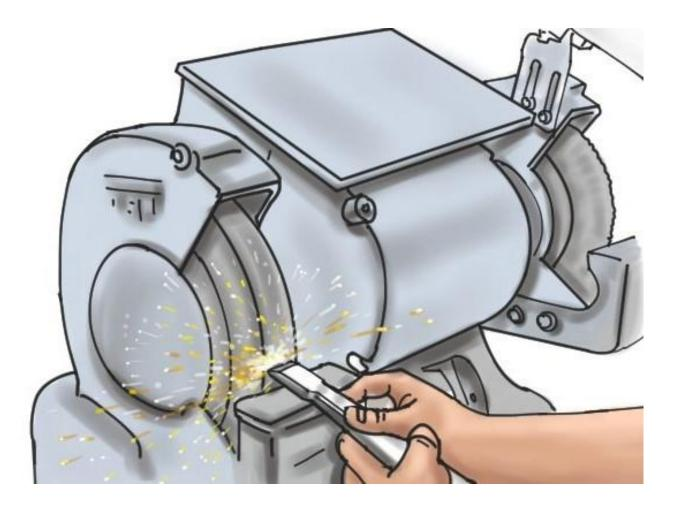
Once the cutting edge has been squared off, the correct cutting angle of 60 degrees will need to be ground into the chisel. As before, only a light pressure with a firm grip should be used to offer the tool to the grinding wheel.
