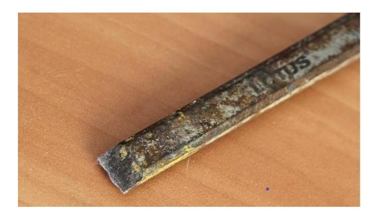
The cutting edge of the chisel is not straight and has been damaged in use. This will need to be ground and sharpened using either the bench grinder or files and whetstone. Using the bench grinder is quicker and easier.
