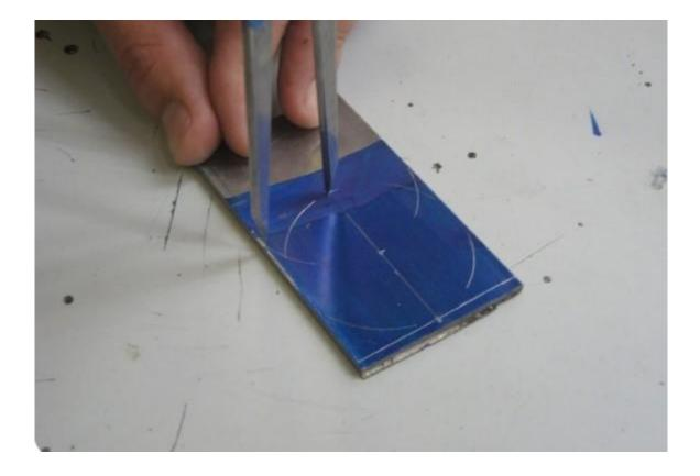
In the diagram the student is using a set of dividers to mark a radius into the Engineer's blue to show where the material will need to be cut. This provides a very fine line and helps to ensure accuracy. The thicker you make the marking the less accurate the cuts will be. Bench-fitting requires precision.
