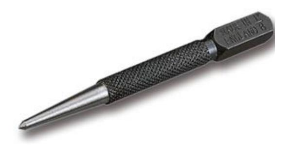
The punch is made from hardened steel, it has a knurled body for grip and a square head to allow it to be stuck firmly with a hammer. The tip is pointed to ensure accuracy when placing onto the work and to allow a small indentation to be made.
