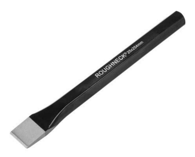
This chisel has a flat cutting edge, these are used for removing excess metal in metal bar or rods, like removing excess wood with a wood chisel. They can also be used for removing sharp burrs or cutting sheet metal that is too thick to cut with tin snips. Another use is to remove difficult rivets or seized nuts and bolts.
