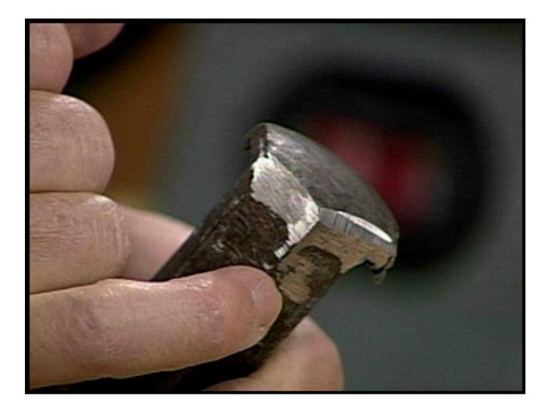
The damage to the head has been removed by using the bench grinder, this has safely removed the mushroom effect.
