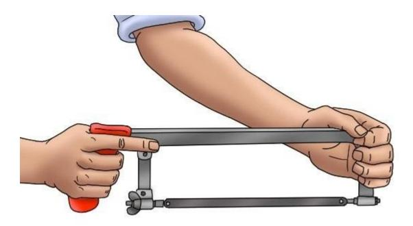
Your feet should be shoulder width apart and you should be stood behind the piece of material that is being cut. You will push the hacksaw with the dominant hand and steady the frame and guide the blade with the other hand. The dominant hand pushes and pulls the hacksaw, the other hand is there to guide and steady the frame to help make a straight and even cut.
