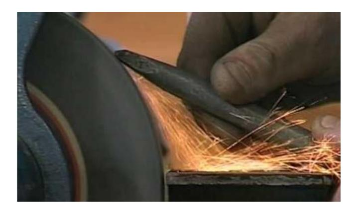
The chisel needs to be offered to the wheel at the correct angle to create the 60 degree cutting angle.
