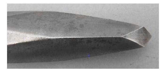
As you can see in the image above, this cold chisel has a specially shaped tip for getting onto sharp corners and areas where other chisels cannot reach. It can be used for removing excess weld or splatter in right angle corners for example.
