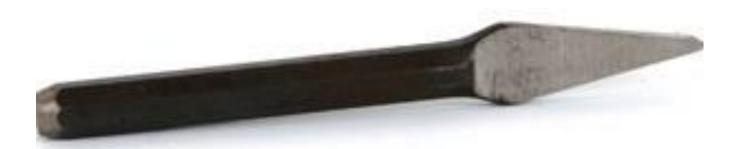
This chisel has a very narrow cutting blade in a diamond shape. This is used to cut a groove or a channel in a piece of metal. The cut would have square edges like a trench.
