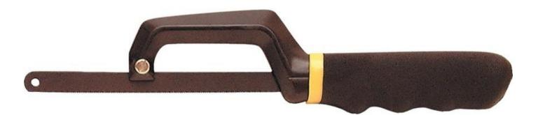
The blade is held inside the hand grip and is secured to the frame with a locking tab shown by the silver screw. The blade extends from the frame and can be used in difficult to reach areas or where a full framed hacksaw cannot be used. This saw uses the 12" hacksaw blades.
